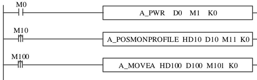
**A\_POSITIONPROFILE指令参数配置**
